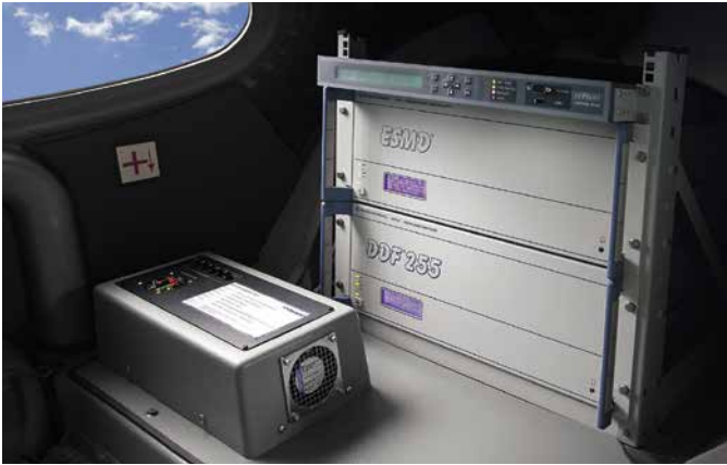
Fig. 4 The R&S®DDF255 digital direction finder and the R&S®ESMD wideband monitoring receiver.
