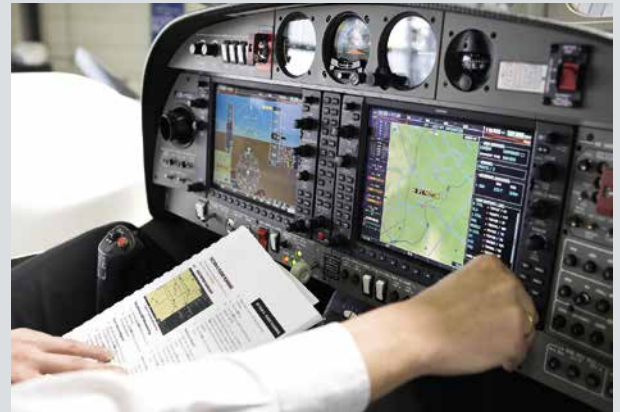
Fig. 1 The flight plan is entered in the flight management system computer.
