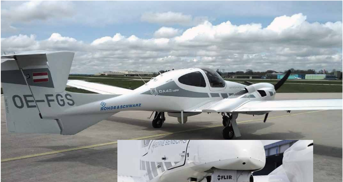
Fig. 3 The aircraft fitted with the DA42M-NG COMINT system (above). In the standard version, the R&S®ADD107 and R&S®HE500 antennas and the FLIR UltraForce 350 camera are mounted externally (right).
