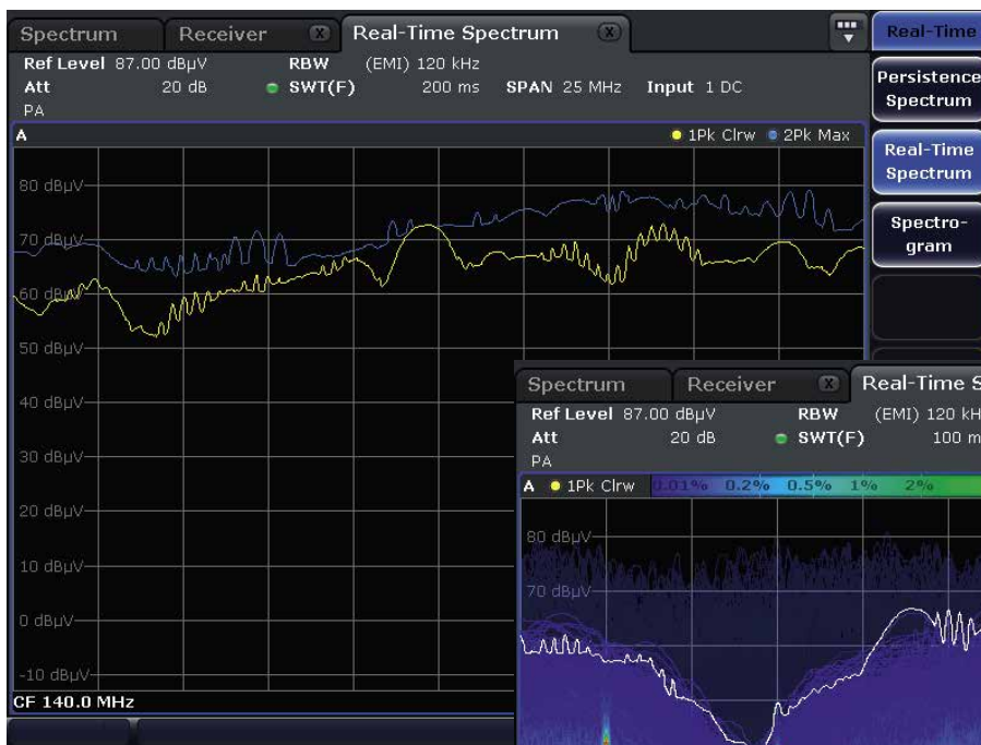
Fig. 5 Display of a broadband disturbance in analyzer mode – in this example caused by an electric motor with poor EMI suppression. The yellow trace represents the current spectrum, the blue trace max. hold.
