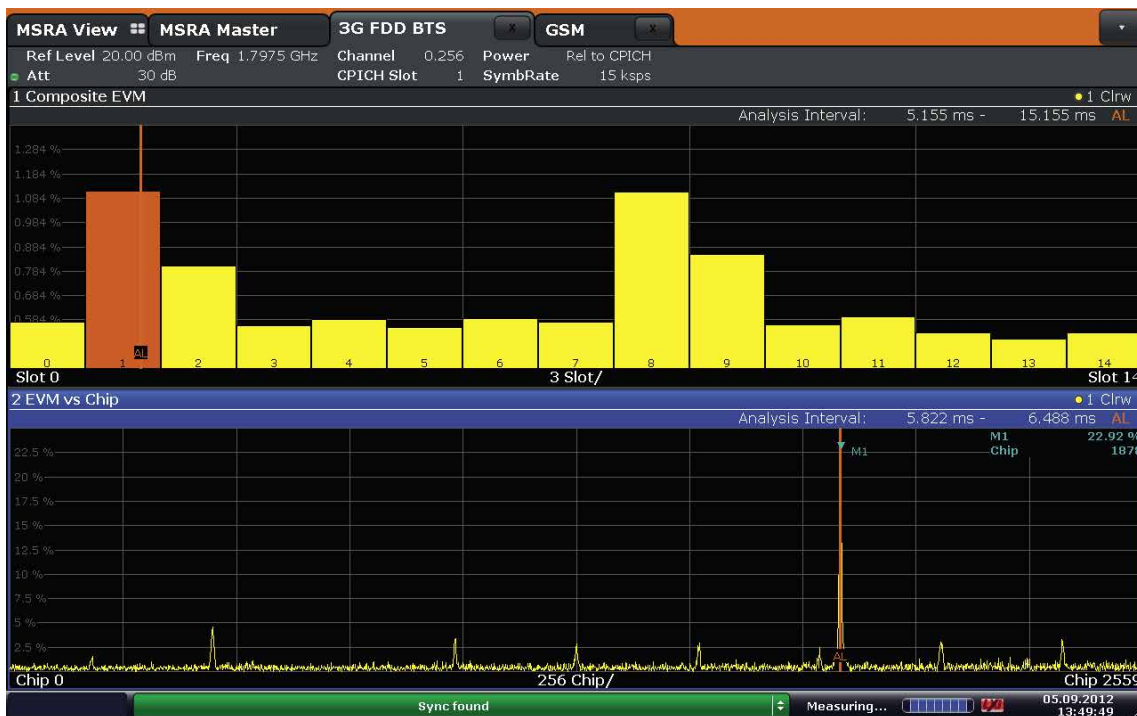
Fig. 3 UMTS measurement showing the Composite EVM and EVM vs. Chip measurements. Slot 1 is highlighted in color in the Composite EVM view (top), and examined in detail in the EVM vs. Chip view (bottom).
