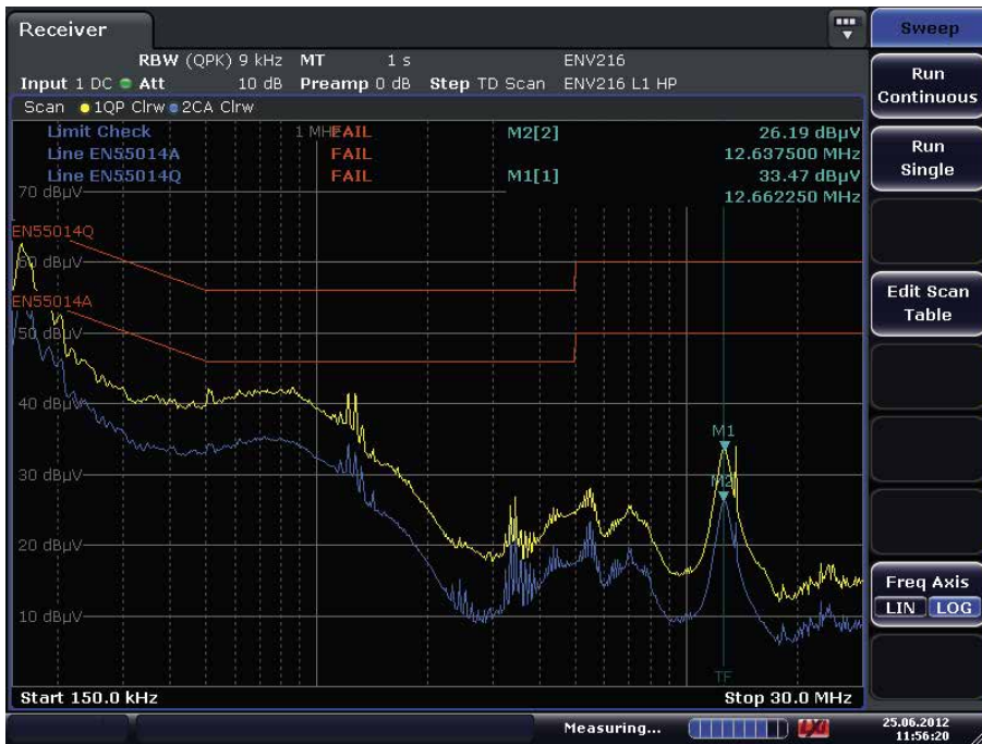
Fig. 3 Disturbance voltage measurement with quasi-peak and average weighting using a realtime time domain scan, plus limit line check with pass/fail indication.
