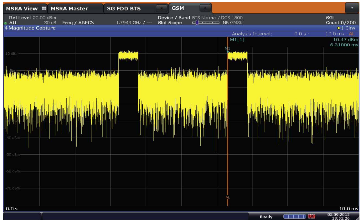
Fig. 4 View of GSM measurement in MSRA mode. The display shows the level versus time. Two GSM bursts are visible. The analysis line is on the rising edge of the second GSM burst.
