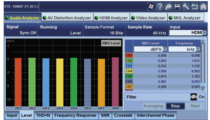
Fig. 6 The R&S®VT-K2150 audio analysis option supports essential audio measurements on the available interfaces.
