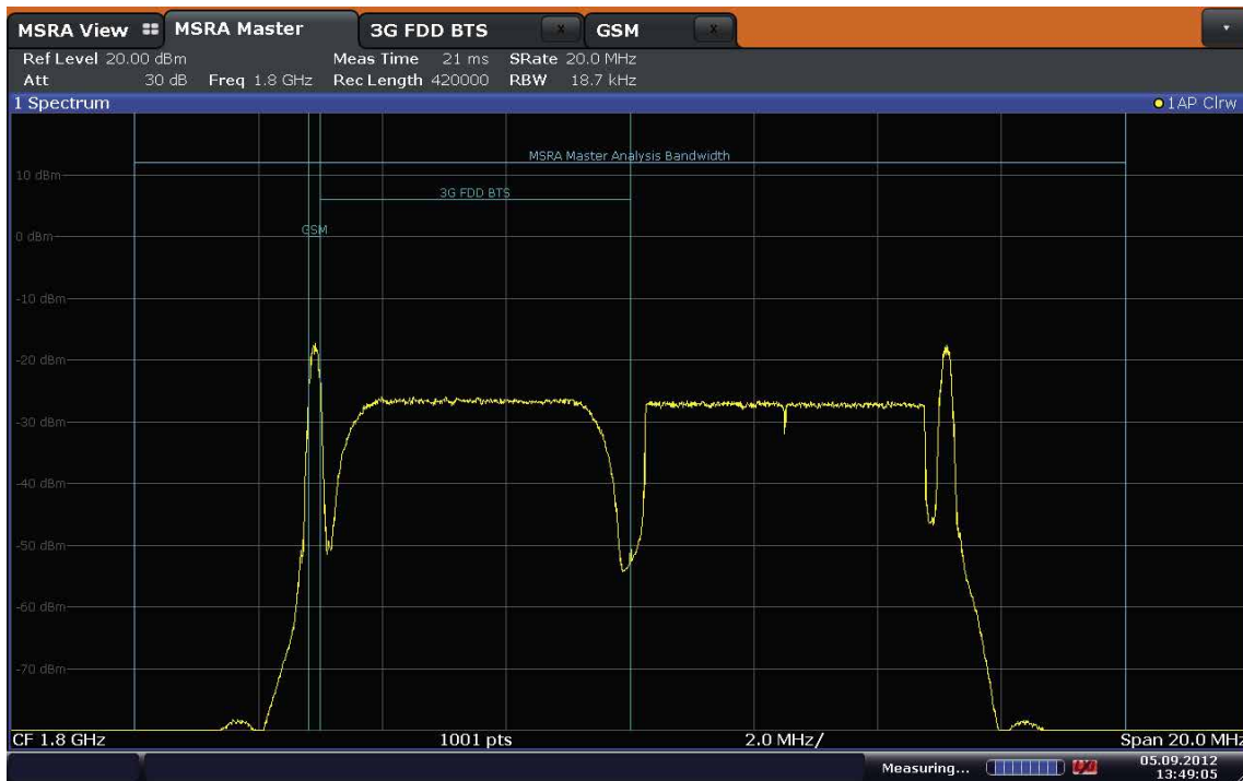
Fig. 2 Display of a multistandard radio signal in MSRA mode; the signal consists of two GSM carriers, one UMTS carrier and one 5 MHz LTE carrier.
